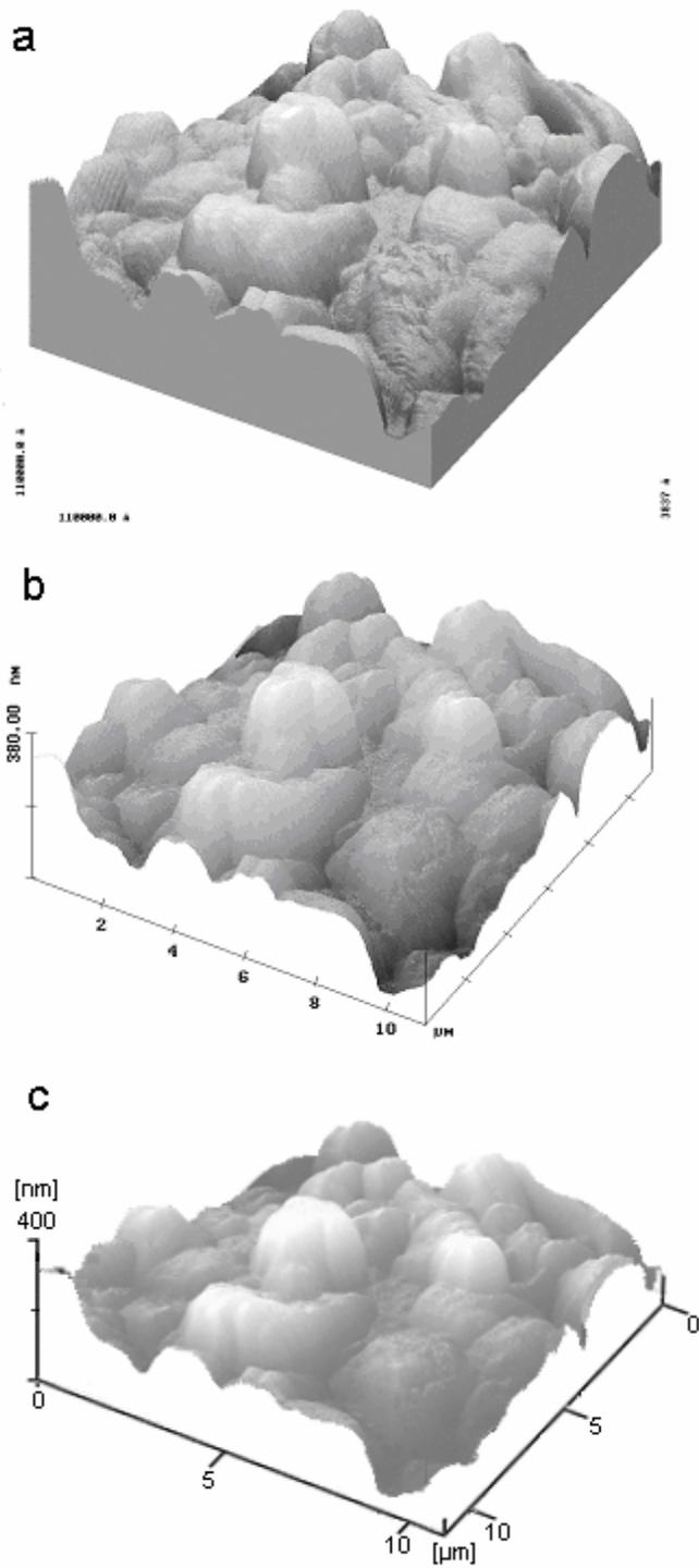
Fig. 4. VRML import from the regular publication [5a]; (a): AFM image of RASTERSCOPE 4000; (b): same image of NANOSCOPE 4; (c): same image of SPI3800N software.
