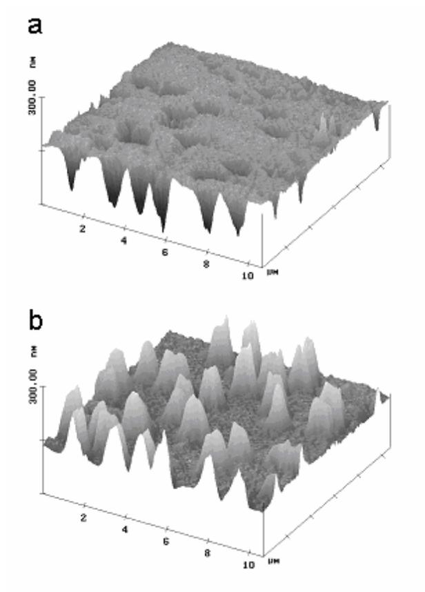
Fig. 8. AFM surface with craters; (a): original; (b): inverted image for the viewing of the crater shapes.
